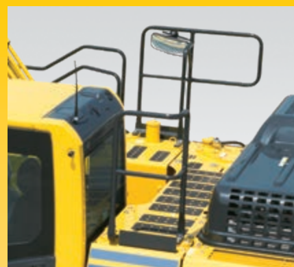
Hand rails and anti-slip plates
