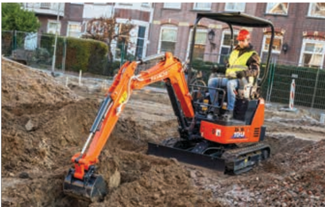
Expandable crawler tracks enhance versatility and stability.
