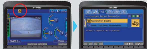
Aftertreatment device regeneration screen
