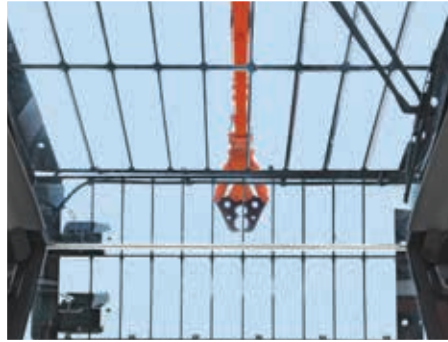
A pillarless window increases upward visibility.
