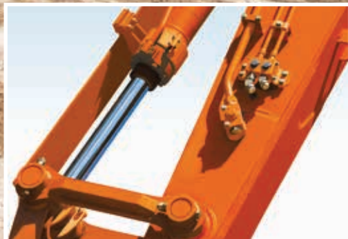
Guard protects the cylinder from potential damage.
