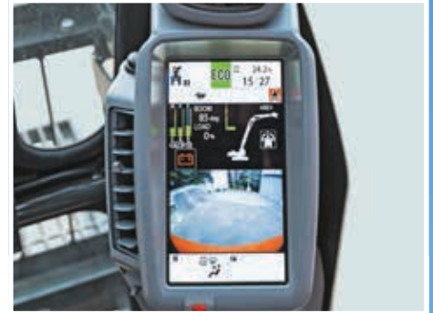
The monitor shows swing angle and overload warnings.
