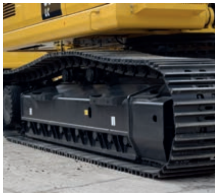
Full length track roller guards (optional)
