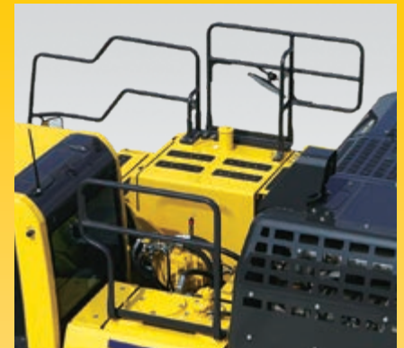
Hand rails and anti-slip plates
